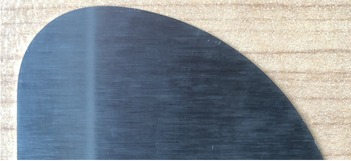
(b) The same part was cut using the proposed method for smoothing the corners.
